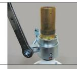
7. Continue winding until the arms meet, use of a ratchet spanner is recommended (18mm)
